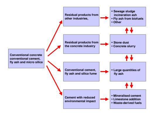
Fig. 1. Overview – concrete developments in the Centre for Green Concrete. New types of cement and binders can be utilised in combination with the residual products.
