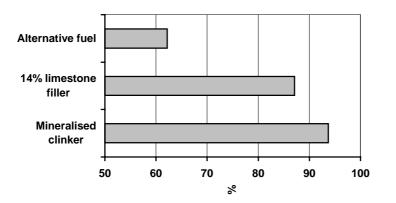
Fig. 2.  $CO_2$  reductions (excl. calcination) expected after present research and development is fully implemented in Aalborg Portland's cement production.  $100\% = CO_2$  emission from Aalborg Portland's largest cements kiln during conventional cement production.
